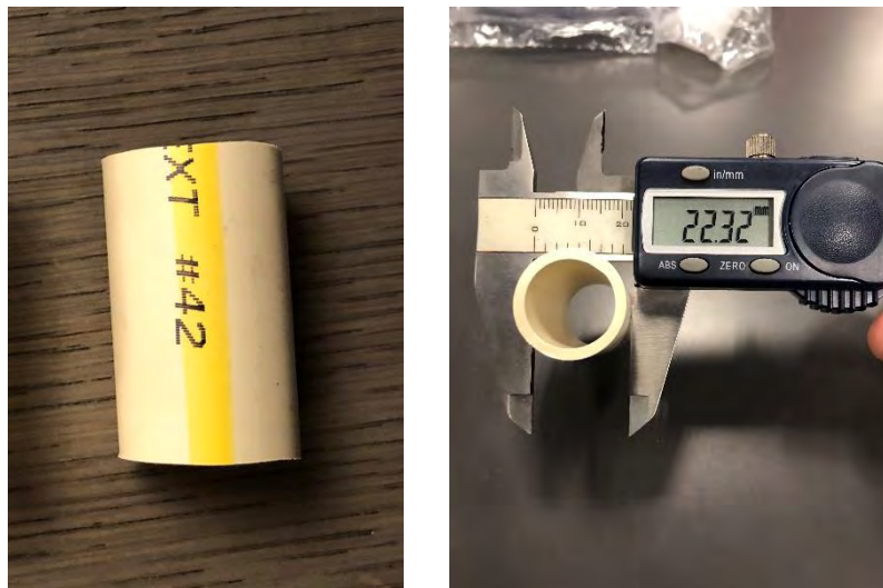
IMAGE 12 - \frac{3}{4} CPVC pipe cut to 4 cm
