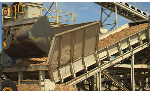
Wood chips loaded on a conveyor belt
