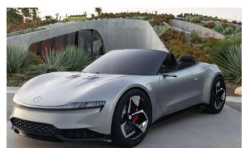
acceleration and driving range. The Rōnin was designed to have three electric motors and designed to provide all-wheel traction and up to 1,000 horsepower. The Rōnin's battery was targeted to provide 600 miles in driving range and the vehicle
