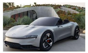
acceleration and driving range. The Ronin was designed to have three electric motors and designed to provide all-wheel traction and up to 1,000 horsepower. The Ronin's battery was targeted to provide 600 miles in driving range and the vehicle
